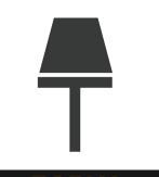
**T-BEAM** 4" x 2" (100mm x 50mm) To 29" x 12" (736mm x304mm)
